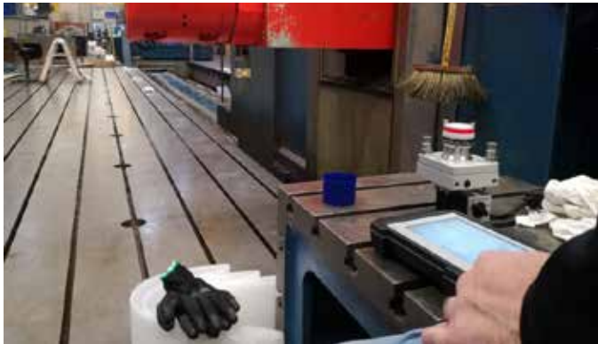
Rectangular flatness across machine foundation.
