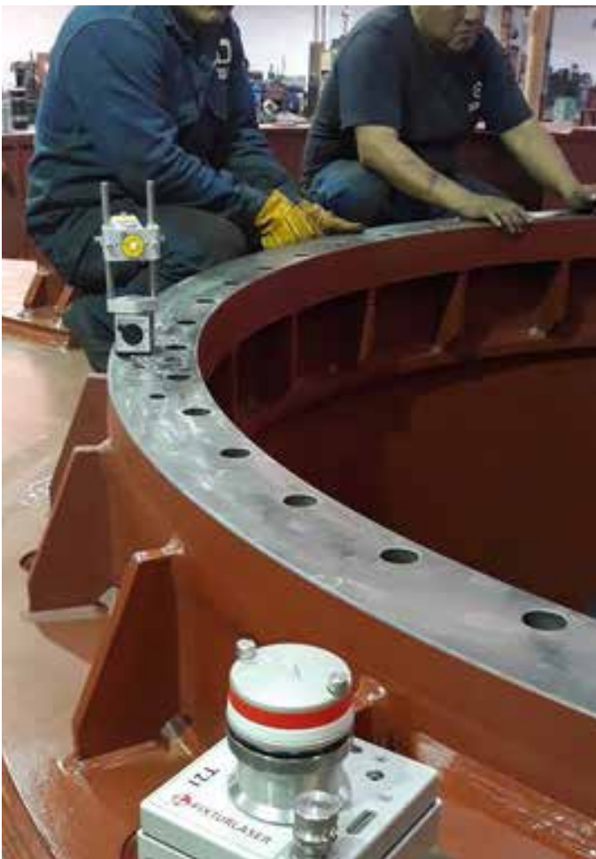
A typical application is the measurement of flanges, e.g. wind turbine towers and machine foundations.
