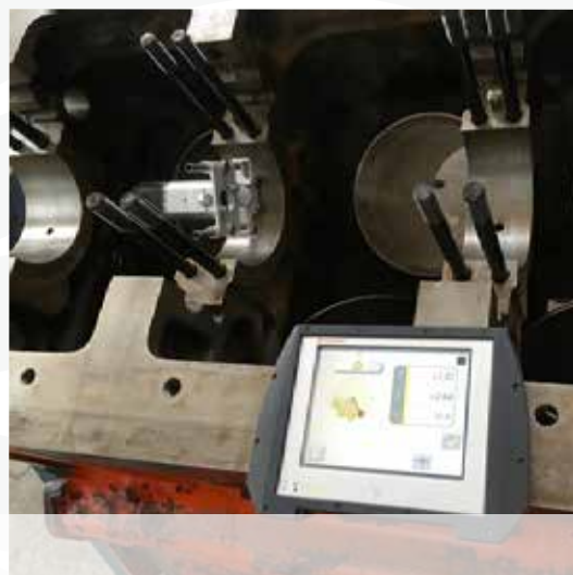
Measurements of bearing journals in split machine casings.
