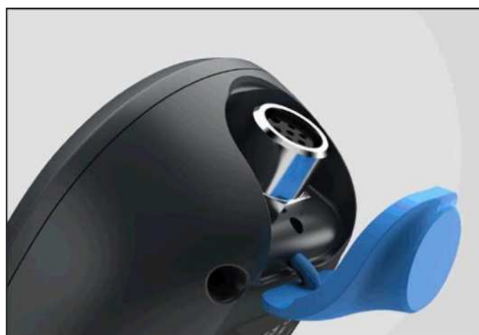
Figure 6 External sensor and charging connector
