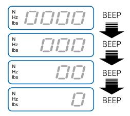
If these signals are seen and heard, batteries should be replaced. Batteries are accessed through the removable cover on the back of the meter. New batteries should be inserted within 30 seconds of removal of old batteries. Taking longer risks loss of any data stored by the memory keys. Batteries are expected to provide approximately 20 hours of continuous operation before replacement is required.
