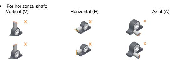
For horizontal shaft and Axial (A), Radial oblique 1 (1) and Radial oblique 2 (2) directions
